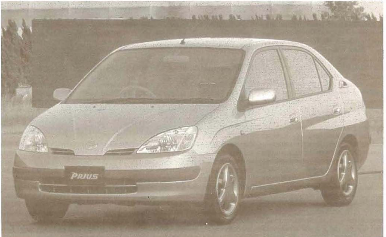
Hybrid auto: The Toyota Prius combines a small combustion engine with an electric generator. Such cars will usher in a "second automobile era," the author argues.
